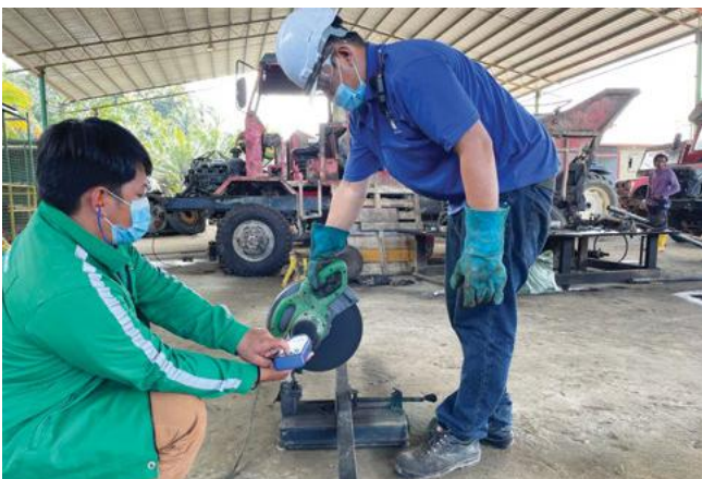
Noise Risk Assessment technician recording sound from metal cutting machine at the workplace
