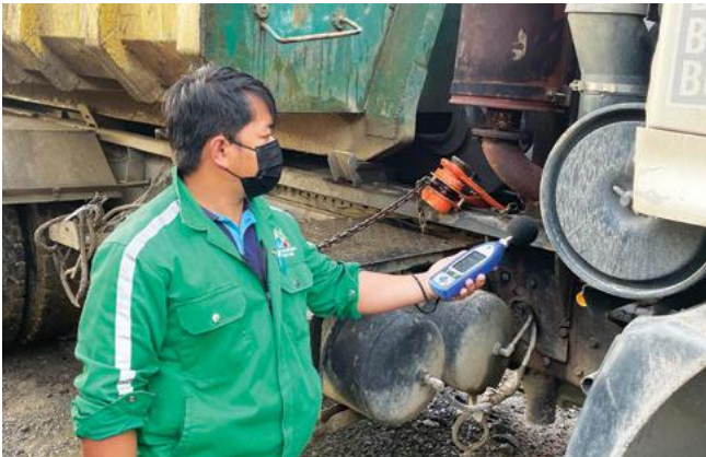
Noise Risk Assessment technician recording sound from the lorry exhaust
