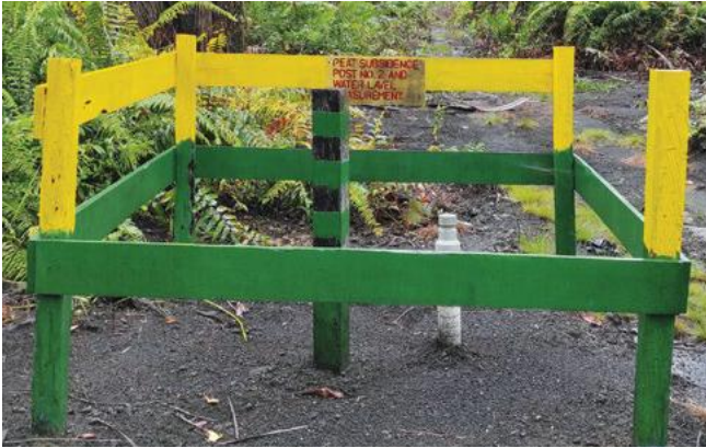
Subsidence post and piezometers installed at peat estates
