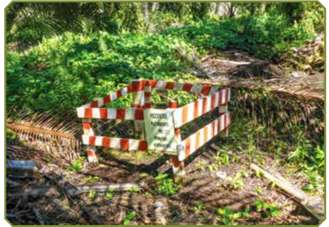
Subsidence posts installed in every peat estate for subsidence monitoring.
