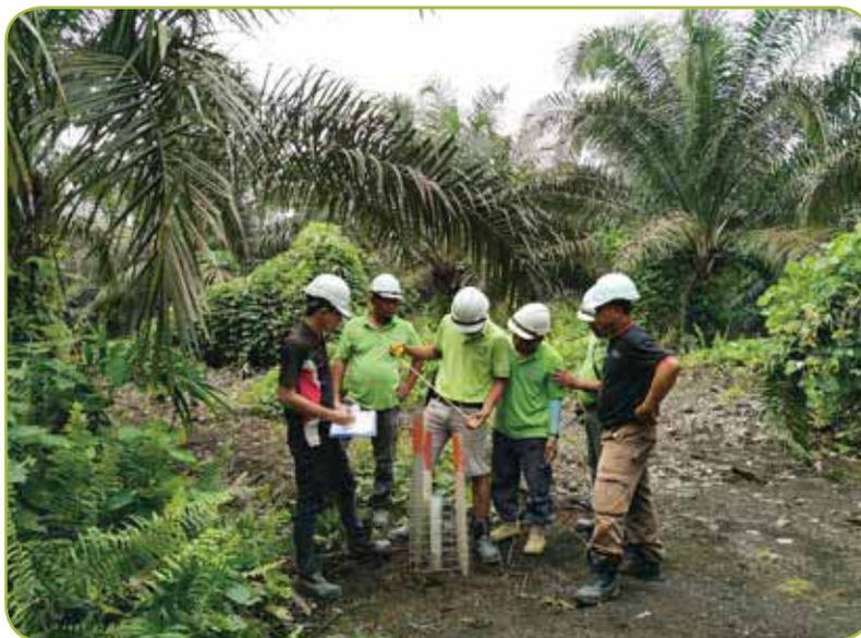
Employees checking the water level using piezometer in Sabaju 3 Estate.
