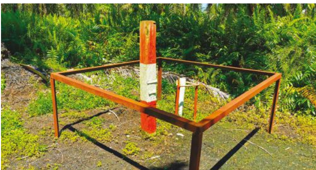
Subsidence post and piezometer installed at a peat estate
