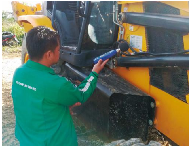
Noise Risk Assessment technician measuring sound from vehicle
